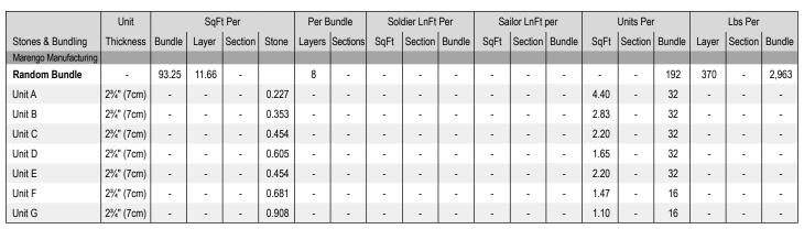
Notes: Sold in full bundles only and is produced and sold on a required, refundable skid. Antique, Smooth and Umbriano finish offer EasyClean™ Stain Resistance technology. Important: A urethane rubber paver mat must be used to prevent scuffing. All measurements are nominal. Contact Unilock for
