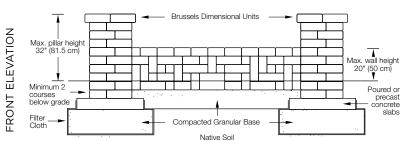
All joints must be adhered with Concrete Adhesive. Base preparation may vary according to soil and climate conditions.
