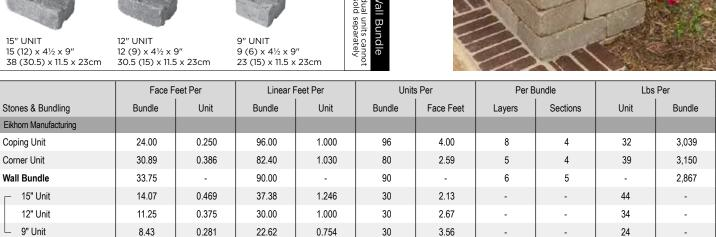
Notes: Structural retaining walls greater than 2' high require professional engineering. Connector units provided with every bundle upon request. Use plastic connectors on set-back walls. Wall Bundle includes 32 End Units per bundle - Not sold separately. Ledgestone", Olde Quarry Coping, Brussels Block' XL, Brussels Fullnose" or 6" x 12" Fullnose complement as a possible coping. All measurements are nominal. Contact Unilock for more information.
